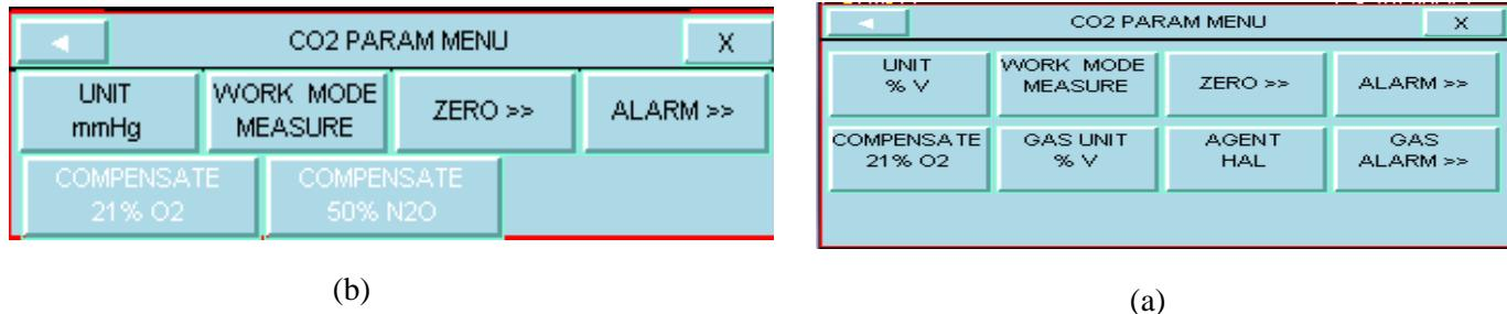
Figure 3-65 a) GAS settings window, b) CO<sub>2</sub> settings window
