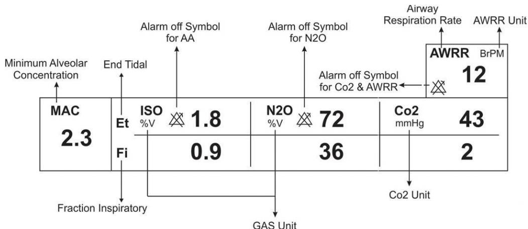
Figure 3-54 GAS parameter area with multi-gas sensor
