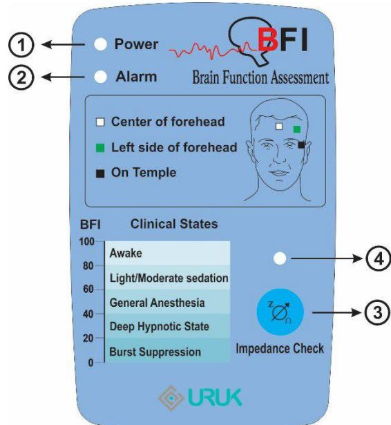
Figure 3-72 BFA module keys and indicators
