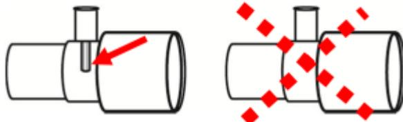
Figure 3-60 For optimal water handling, always use T-adapters with the sampling point in the center of the adapter, as shown to the left above.
