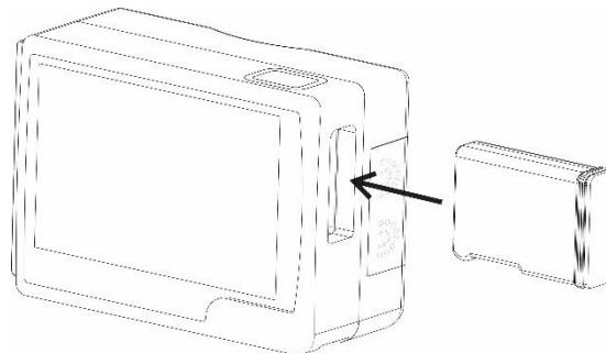
Figure 1-7 Battery insertion
