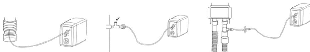
Figure 3-61 Analyzer placement in respiratory circuit
