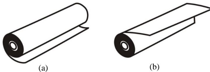
Figure 2-13 Paper placement a) incorrect, b) correct
