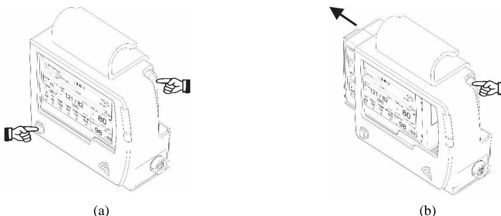
Figure 1-6 Removing PM4010 from the station
