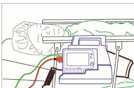
Figure 1-11 PM4010 connected to the edge of bed
