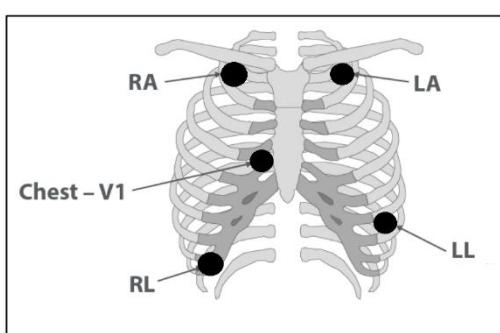
Figure 3-3 Electrodes' locations for 5-wire ECG cable
