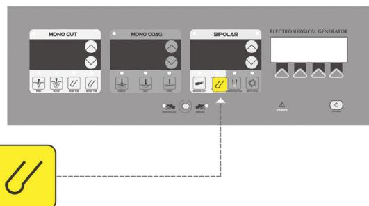
At Bipolar TUR, The Bipolar output power can be increased up to 250 Watts. So Cutting in Normal Saline is available
